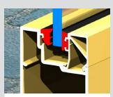
We offer security glazing as shown above. Captive co-extruded glazing wedge on the outside. We can use silicone wet top on the outside in lieu of the captive wedge.
